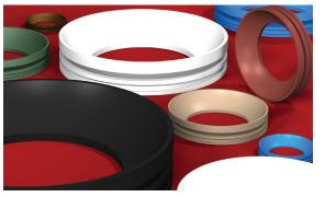
Because virgin PTFE has lower physical properties than other filled PTFE materials, it is not recommended for use in applications where fluids are abrasive or contaminated with small particles. Abrasives can wear down the material and cause leaks to occur.
